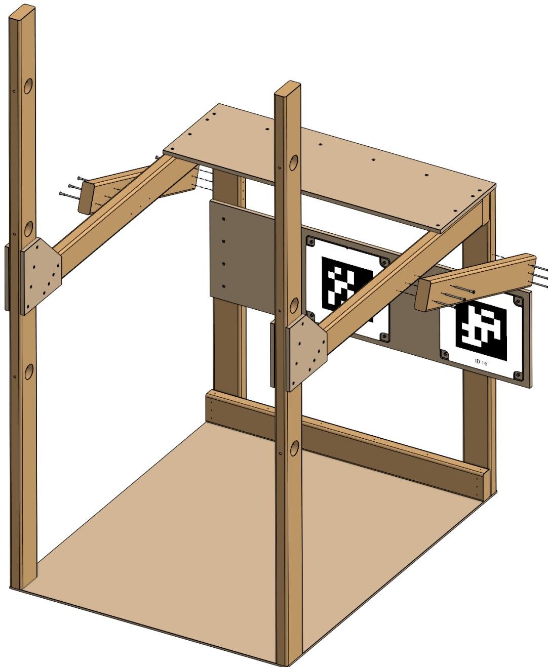
6. Slide in all three TE-26509s (Tower Rung) into the TE-26502 (Tower Upright Beam) and fix them in place by using the 1/4-20 x 4" Long Bolt Hex Bolt with Lock Nuts through the Rung. The ends of the rungs should extend 5-7/8in beyond the outside edges of the TE-26502 (Tower Upright Beams).
