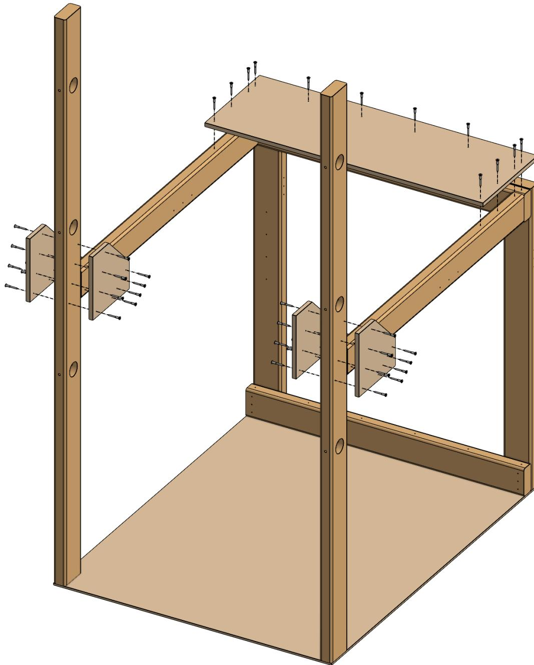
4. Attach the TE-26510 (Tower April Tag Plate) to the inside of both TE-26504s (Tower Vertical Support Beam) and keep it flush with the left Vertical Support and mount it 15-13/32in above the TE-26501 (Tower Bottom Base Plate). All using 1-1/2in screws.
