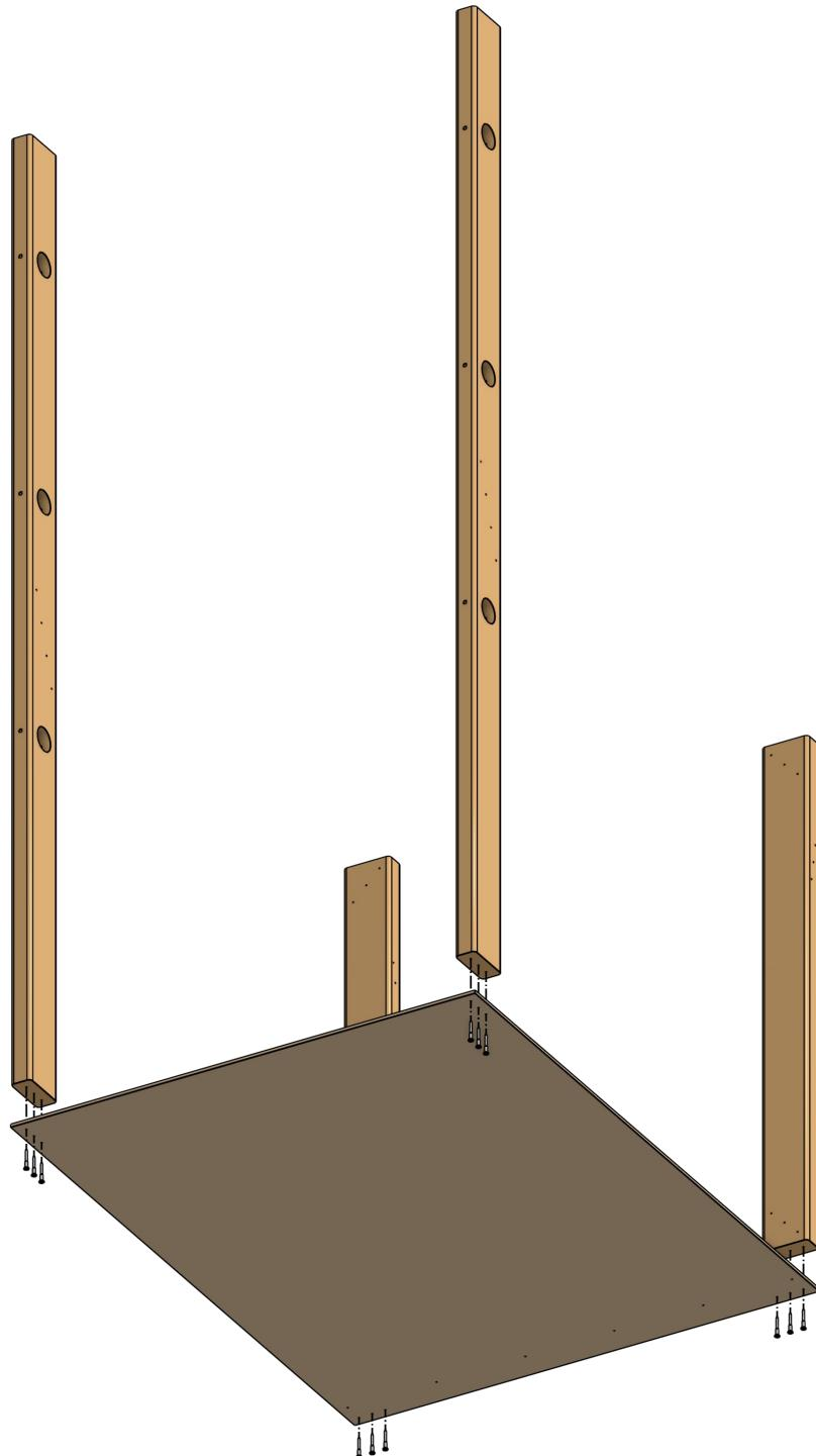
2. Attach both TE-26505 (Tower Horizontal Support Beam) to the top and bottom of the TE-26504s (Tower Vertical Support Beam) using 2-1/2in screws and to the top of the TE-26501 (Tower Bottom Base Plate) using 1-1/2in screws.
