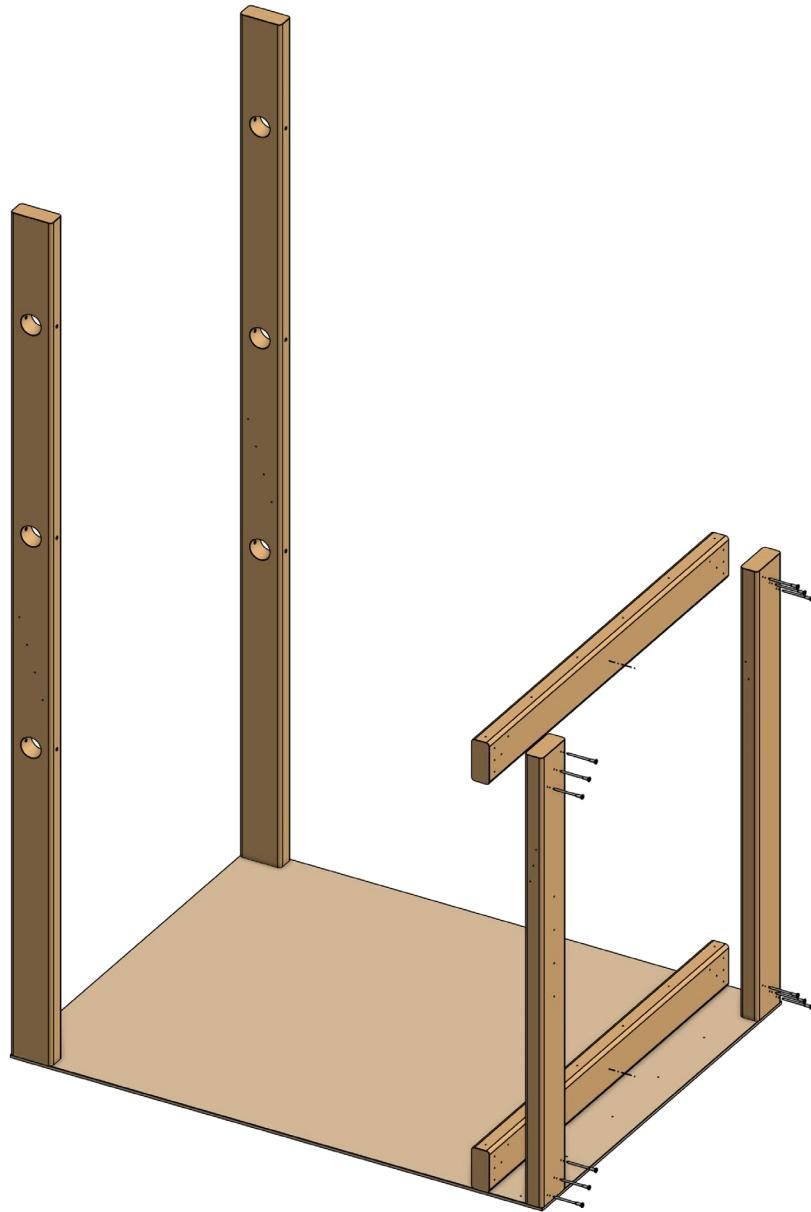
3. Attach both TE-26503 (Tower Upright Support Beam) using 4 TE-26508 (Tower Upright Support Plate) on both sides of the TE-26502 (Tower Upright Beam) and the TE-26507 (Tower Top Support Plate) on top of the TE-26505 (Tower Horizontal Support Beam). The bottom of TE-26503 should be 34-3/4in from the bottom of TE-26502. Fasten all using 1-1/2in screws.
