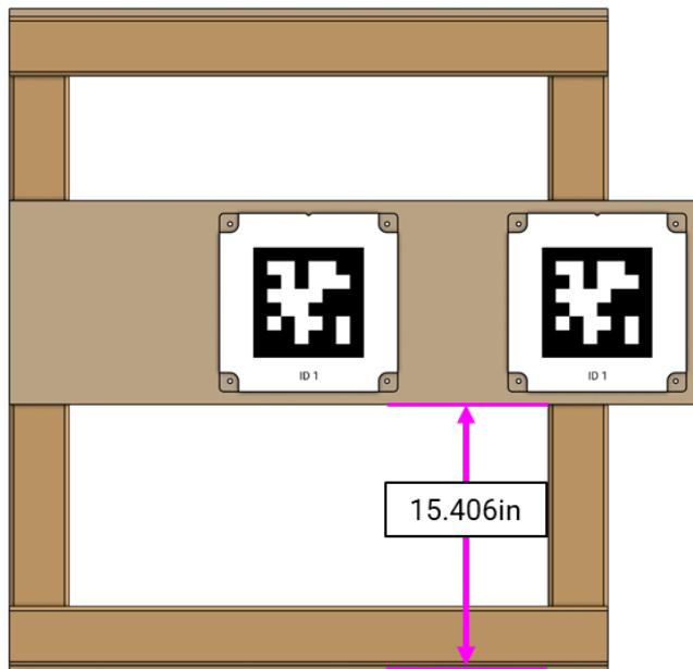
5. Attach two TE-26506s (Tower Angle Support Beam) approximately halfway down the outside of each TE-26503 (Tower Upright Support Beam) at a downwards angle touching the top of TE-26510 (Tower April Tag Plate). Attach using 2-1/2in screws.
