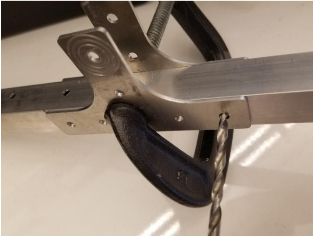
Figure 7: Clamping T-Brackets to Bar
