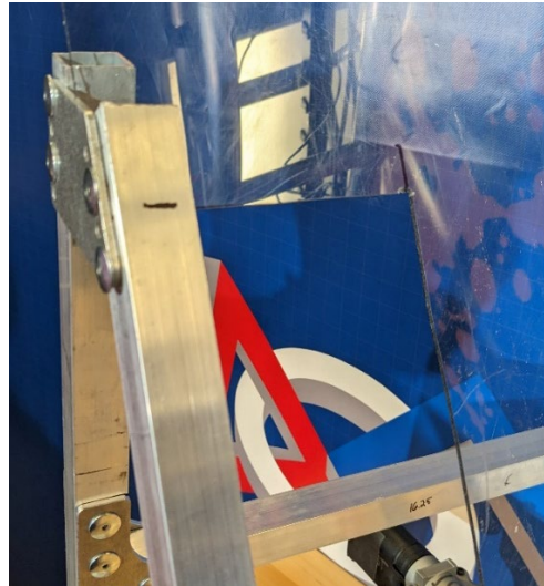
Figure 28: Marquage du tube diagonal
