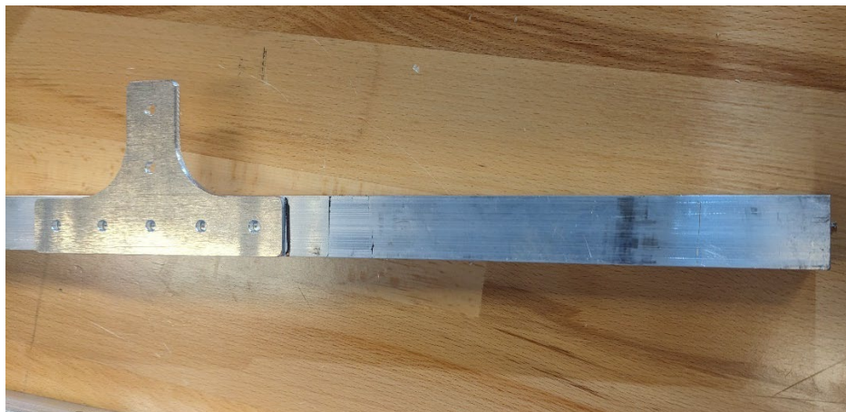
Figure 6: Placement correct du support en T
