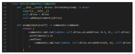
Our example file only has a single autonomous routine to get. You could easily extend this pattern by adding additional methods to define more autonomous routines and you <u>could select between them</u> <u>using a SendableChooser on the dashboard</u>.
