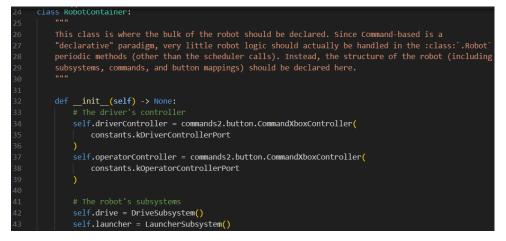
The first section of the constructor sets up some member variables in the class. For RobotContainer this generally includes all of your subsystems and control devices. This code uses the CommandXboxController class to represent the gamepads as it contains a number of helper methods that make it much easier to connect commands to buttons.
