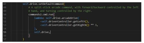
Another common modification is to scale the values down by default, but allow for the maximum value if a button is pressed (turbo mode). This type of modification can also be done at the point of capture, though as complexity grows, you may wish to shift from an inline command definition to a different type where you can define the command behavior more clearly.
