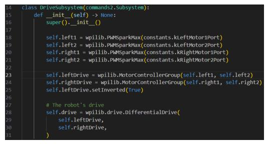
The first line of this image is the class declaration. This declares the name of our class and says that it's an extension of the Subsystem class. All subsystems should extend this class which provides some utility functions regarding setting the name of the subsystem, registering it with the scheduler, and sending information about it to the dashboard.
