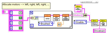
In the next Enable/Disable structure (disabled by default) is the code for setting up the drivetrain if you have connected your motor controllers over CAN. If you have not installed REVLib properly, or not restarted LabVIEW since installing, these icons will show as '?' symbols. This code functions very similar to the PWM drivetrain code described above, but it explicitly sets the motor type to 'Brushed' to match the CIM motors used on the KitBot and sets a 60 Amp current limit on the motors.
