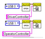
This code from the top center of the diagram opens a reference to a controller connected to ports 0 and 1 on the Driver Station and saves those references to RefNums called DriveController and OperatorController respectively.
