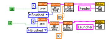
The CAN Launcher code opens a reference to the SPARK MAXs, and sets them to be inverted. This was needed on our KitBot to make the wheels spin outward (launching) with a positive command and inward (intaking) with a negative command. If your robot behaves differently, you can either modify these inversion constants or negate the values used in the launcher control. This code also sets the current limit on the motors to the default value of 80 Amps.
