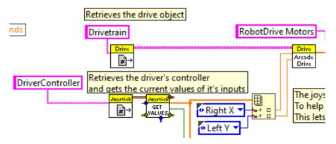
This section of code accesses the joystick values from the DriverController, selects the value of specific axes from the axis array, and uses those values to control the drivetrain in Arcade Drive. Arcade Drive controls the robot rotation with one value (here the Right X axis value) and the robot speed with a separate value (here the Left Y axis value).
