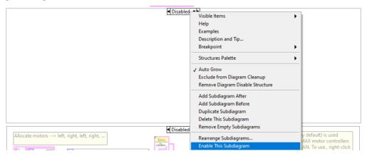
The top block of code for PWM control is Enabled in the project by default. Click the arrow next to "Enabled" to switch to the empty Disabled case, then right-click and select "Enable This Subdiagram". This will disable the PWM code and enable the blank diagram.
