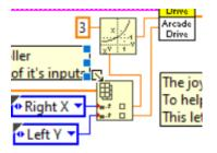
Another common modification is to scale the values down by default, but allow for the maximum value if a button is pressed (turbo mode).
