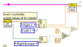
Example: Scale the forward-back driving by 50% unless the right bumper is pressed
