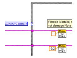
In the Intake portion of the case structure, the Launcher wheel is set to run inwards at max speed and the Feeder wheel is set to run inwards at a low speed. This pulls the Note in fully, but avoids rapidly grinding the wheel against the Note once it is fully inside the robot.
