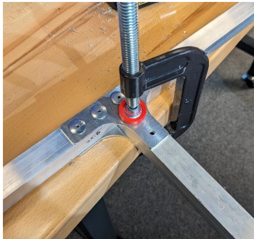
Figure 9: Securing the Horizontal Tube
