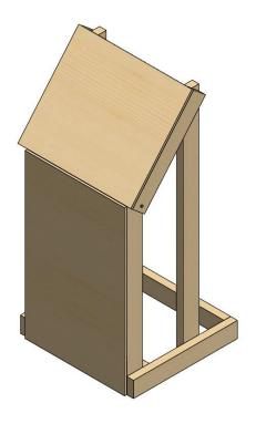
**Description:** This is a Source, designed so that teams can practice acquiring game pieces. Three of this assembly can be placed side by side to replicate a full width Source. If combining three of these assemblies, consider adding thin walls between them to simulate the dividers in the Source assembly.
