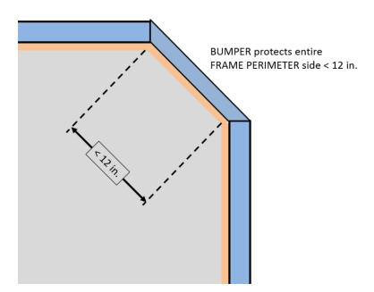
Figure 9-3 BUMPER around full side/corner
