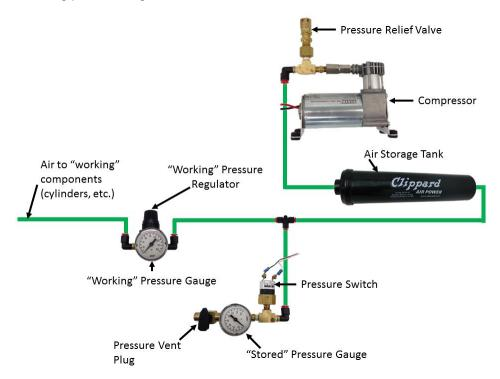
Figure 9-15 Pneumatic circuitry
