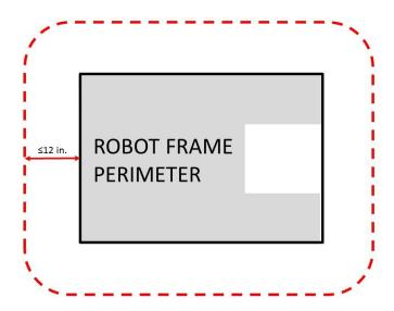
Figure 9-1 FRAME PERIMETER extension
