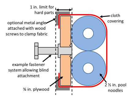
Figure 9-7 BUMPER vertical cross section
