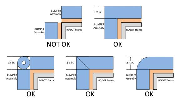
Figure 9-8 Soft parts of BUMPER corners
