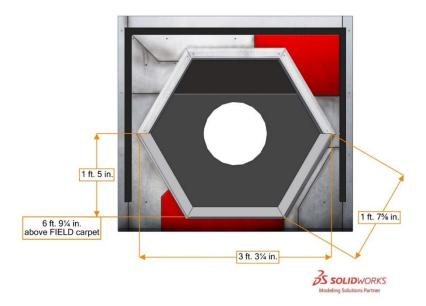
Figure 3-26 POWER PORT vision target
