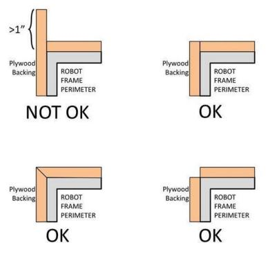
Figure 9-5 Hard parts of BUMPER corners
