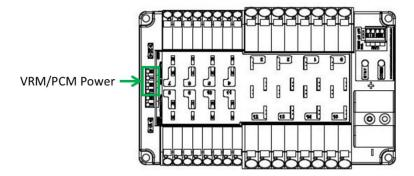
Figure 9-13 VRM and PCM power source
