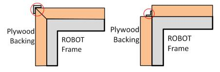
Figure 9-6 Hard parts of BUMPER corners
