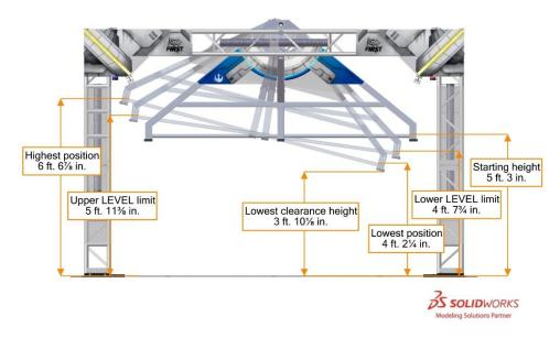
Figure 3-9 GENERATOR SWITCH range of motion (note: dimensions are to the top of the floor protection carpet)
