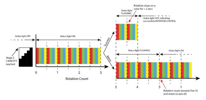
Figure 3-24 CONTROL PANEL ROTATION CONTROL example
