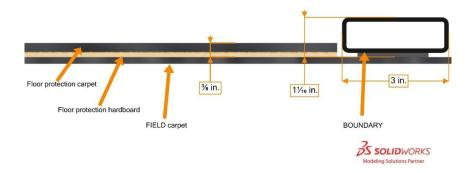
Figure 3-11 Floor protection cross-section
