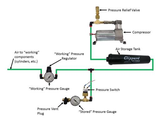
Figure 9-14 Pneumatic circuitry
