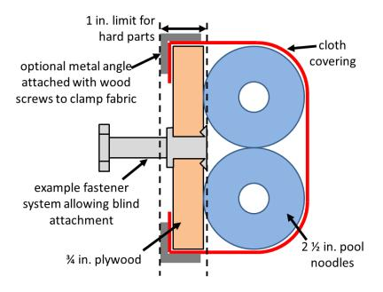
Figure 9-6 BUMPER Vertical Cross Section
