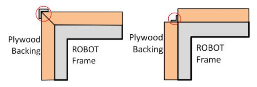
Figure 9-5 Hard Parts of BUMPER Corners
