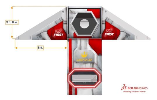
Figure 3-16 Backboard dimensions
