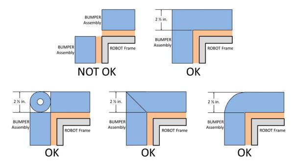
Figure 9-7 Soft Parts of BUMPER Corners
