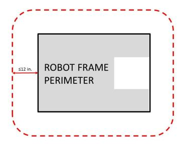
Figure 9-1 FRAME PERIMETER extension
