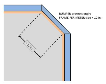
Figure 9-3 BUMPER around full side/corner.
