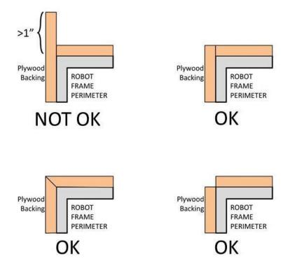
Figure 9-4 Hard Parts of BUMPER Corners
