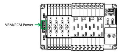
Figure 9-12 VRM and PCM power source
