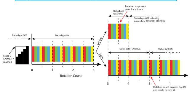
Figure 3-24 CONTROL PANEL ROTATION CONTROL example
