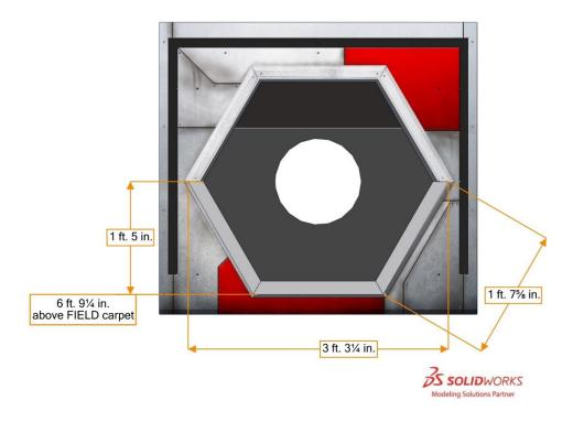
Figure 3-26 POWER PORT Vision Target
