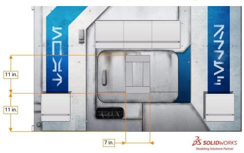
Figure 3-27 LOADING BAY Vision Target
