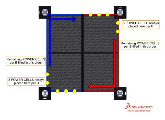
Figure 4-2: POWER CELL setup on BOUNDARIES
